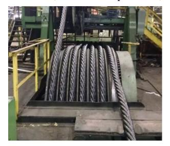
Finally, we come to the heart of the factory: We stand, astonished, gazing up at the 12 foot tall, 800 tonne closing machine, designed to produce the 7 inch rope for dragline boom pendants, and construction cable like that used to build the Brooklyn Bridge. The already huge strands are all dragged into a central point, slowly weaving the helical pattern of wires around a hefty centre rope into a single massive cable which will one day end up on a dragline somewhere in the world.
